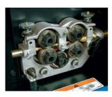
Industrial 4roll gear-driven cast aluminium drive system & heavy-duty motor provides wire speeds ranging from 0-20m/min. Available with Euro style or US Style torch connections offering exceptional feed performance & reliability.
