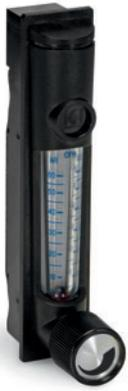
**Gas Flowmeter Kit #246 127** Field Monitors and adjusts gas flow at the feeder.
