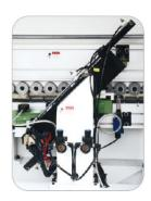
End-trimming mechanism through a precise guide track movement, adopt automatic tracking and high-frequency motor fast cutting structure to ensure the cutting surface smoothly.
