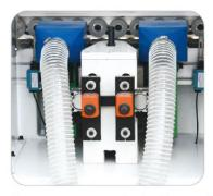
Trim equipment with double trim-blades works on the waved effect that is caused by precise dimersicen saw.
