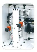
Scraping unit for a perfect finishing of the applied edge.
