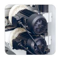
The buffing device adopt the board processed by cotton poloshing wheel, by end poloshing to make a more smooth surface.
