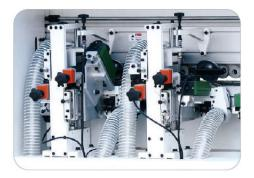
Rough/Fine trimming mechanism used for repairing the excess edge materials, adopt automatic tracking and high-frequency motor fast cutting structure to ensure the trimming plates smotthly.
