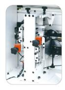
Scraping unit for a perfect finishing of the applied edge.
