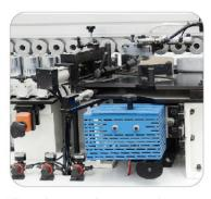
The glue mechanism adopt a special structure to gelatinize the plates and coating materials uniformly, ensure a more solid conglutination.
